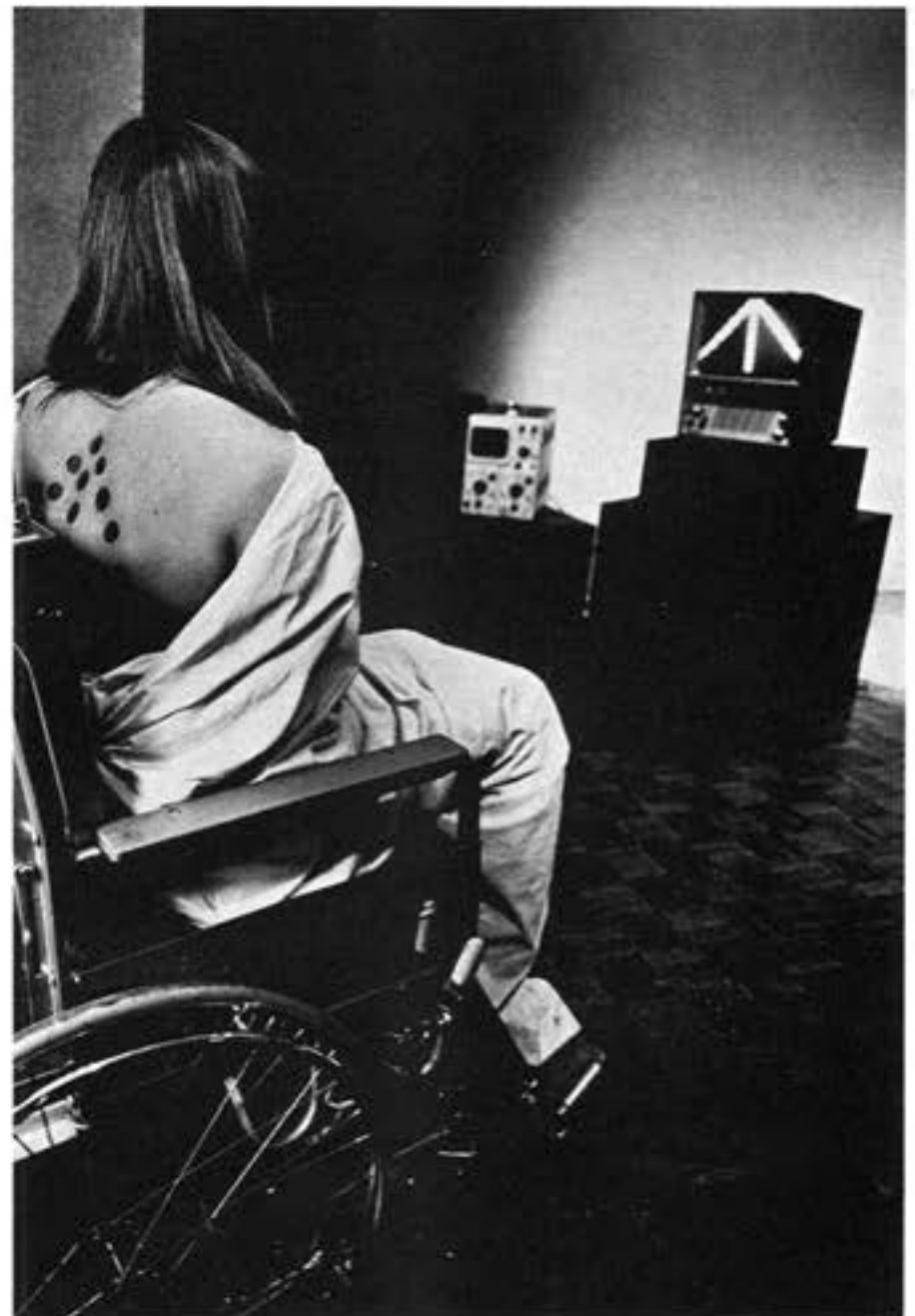
The tactile image, simulated here on the seated girl's bare back, corresponds to the visual image on the screen.
