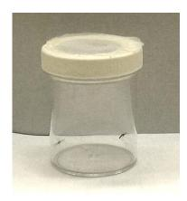
Figure 3.7.3.1. This particular choice of tube that we use for family oviposition is modified from a chamber purchased through Qorpack (Bridgeville, PA. No. 3891). Many similar tubes are suitable. The bottom may be covered with a filter paper disk to absorb fluids.
