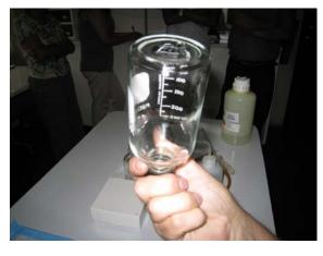
Figure 5.1.3.4: Coating the top of the bottle
