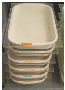
**Figure 1.4.4.** Different colors of tape and/or different colors of markers make it obvious to see the difference between stocks at a glance. They also make it simple to locate material rapidly.
