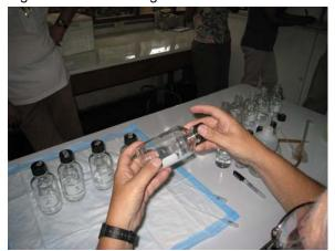
Figure 5.1.3.5: Coating the sides of the bottle
