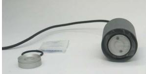
**Figure 2.4.10.4.** The electric heating unit with a membrane feeder attached to the bottom.
