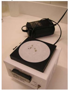
**Figure 3.4.2.** A small Peltier cold table on which damp filter paper is placed to conduct cold and prevent mosquitoes from sticking to the condensation.
