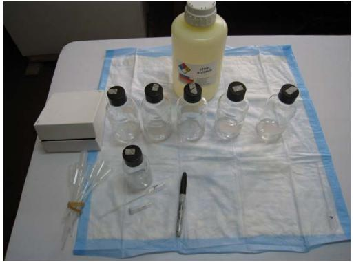
Figure 5.1.3.1: Material and reagents for the CDC Bottle bioassay
