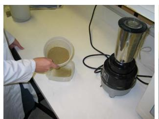
**Figure 2.4.6.1.** Preparing food. Use a general laboratory grinder (pictured here), a grinding mill or a household coffee grinder. To ensure food is small enough for the earliest stages, use a sieve with holes no larger than 250 microns in size.
