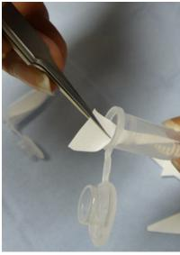
**Figure 3.8.2** Inserting the filter paper triangle
