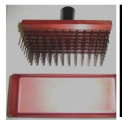
**Figure 3.5.1.** Example of a 96-bacterial replicator tool used for maceration of mosquito samples and reservoir.
