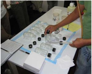
Figure 5.1.3.7: Transferring mosquitoes into insecticide-coated bottles
