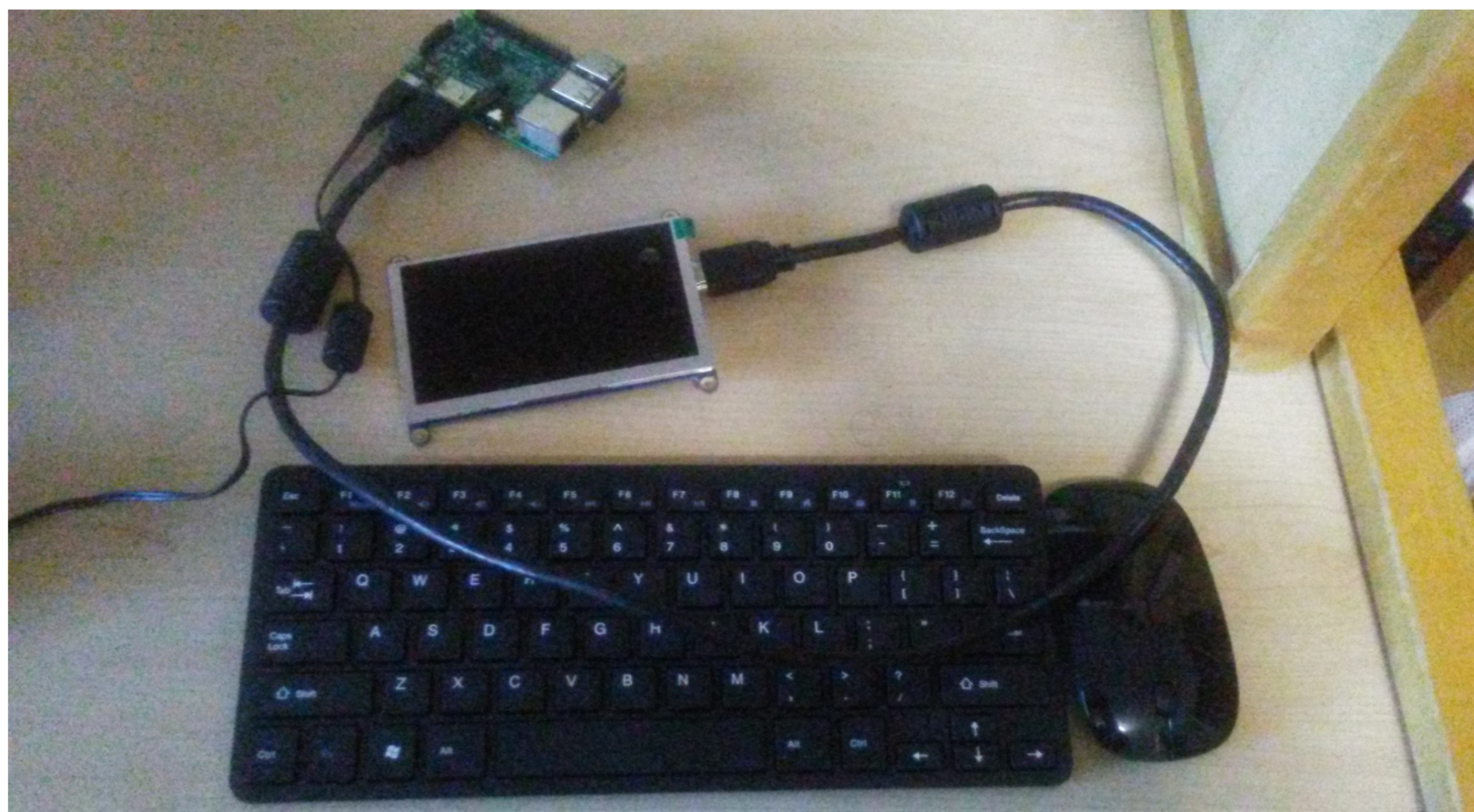
Figure 1: The figure above shows an LCD screen connected to a Raspberry Pi 3 (RasPi3) which serves as a microcontroller or a mini computer. We will use the LCD screen to primarily insert our code into the RasPi3. Once implementing our code, we will utilize the LCD screen as a form of visual alert for the user.
