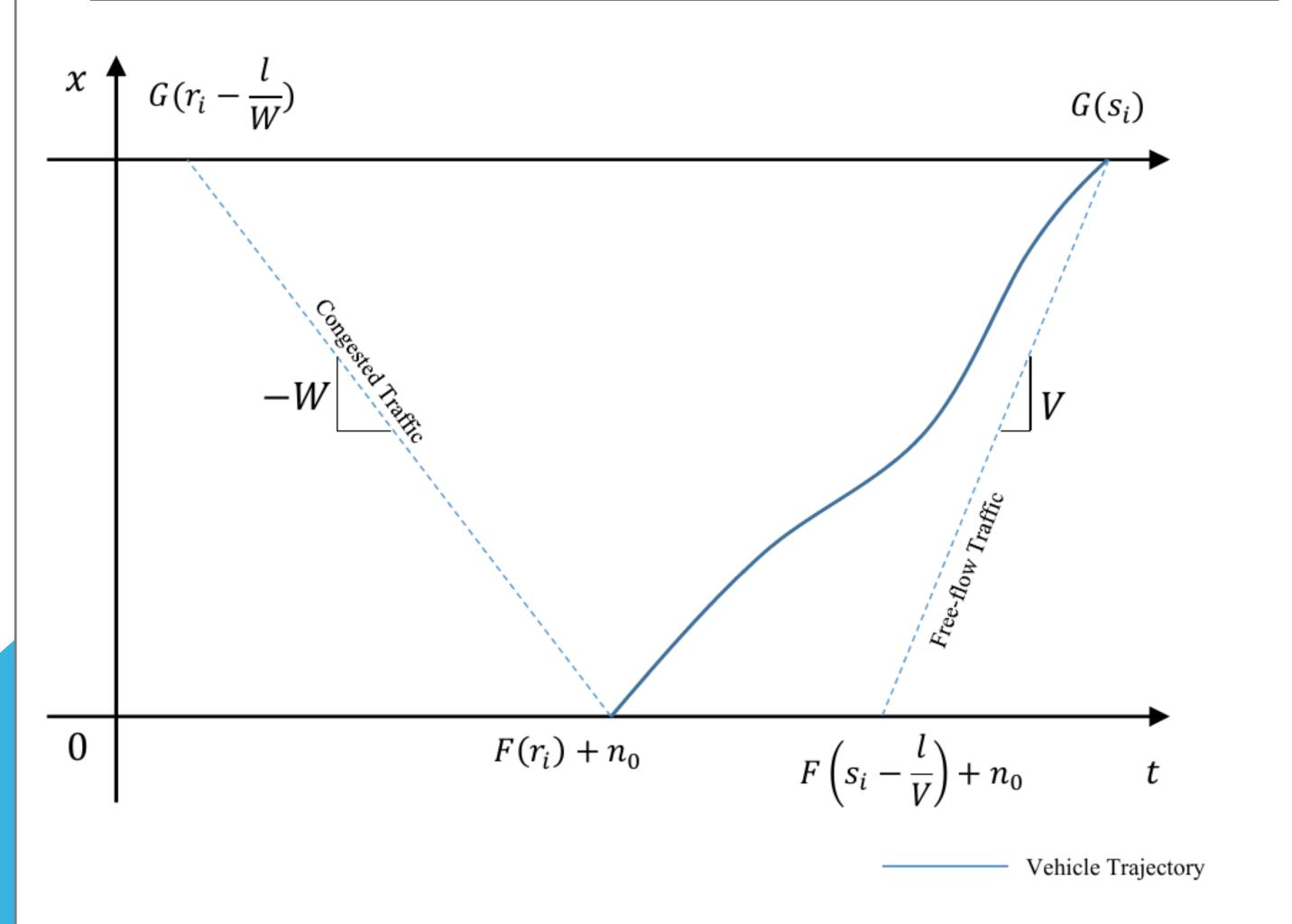
In the above plot, the solid line is the trajectory of vehicle i and the dash line is the backward traveling wave. The FIFO assumption leads to
