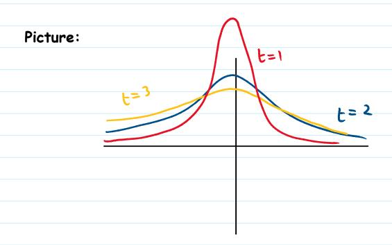
3) To solve  $u_t = k u_{xx}$  replace t by kt to get that the fundamental solution is:
