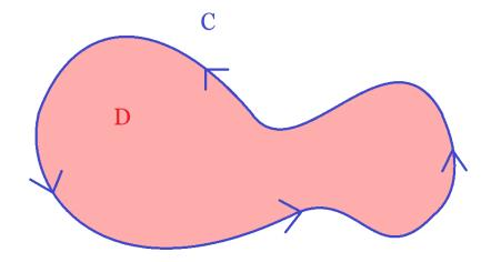
The idea is that instead of calculating a hard line integral (left), you calculate an easier double integral.
