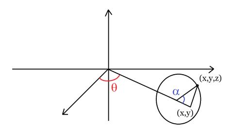
$\theta$  = angle between x-axis and  $(x,y)\alpha$  = angle between (x,y) and (x,y,z)
