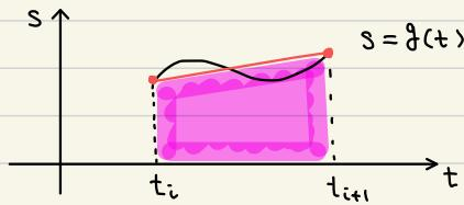
$$\int_{t_i}^{t_{i+1}} g(t) dt \approx \frac{h}{2} (g(t_i) + g(t_{i+1})) \\ = \frac{h}{2} (f(t_i, y(t_i)) + f(t_{i+1}, y(t_{i+1})))$$
