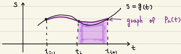
$$\Rightarrow w_{i+1} - w_i = \int_{t_i}^{t_{i+1}} at^2 + bt + c dt$$
