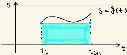
$$\begin{aligned} \int_{t_i}^{t_{i+1}} g(t) dt &\approx (t_{i+1} - t_i) g(t_i) \\ &= h f(t_i, y(t_i)) \end{aligned}$$
