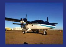
DHC-6 Twin Otter – Twin Otters are among the most versatile airplanes in NOAA's fleet. They can carry many different payloads and be configured to support multiple mission types, from marine mammal and snow surveys to coastal mapping and oil spill response. These short-takeoff and-landing aircraft can operate where many other aircraft cannot. NOAA currently operates four Twin Otters.
